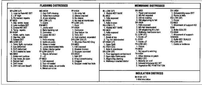
Figure 2 Abbreviated list of flashing, membrane and insulation distresses.
