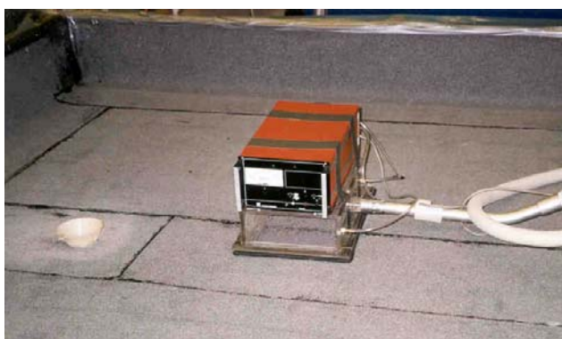
Figure 4: Pressure box with tracer-gas detector and connected air pump.
