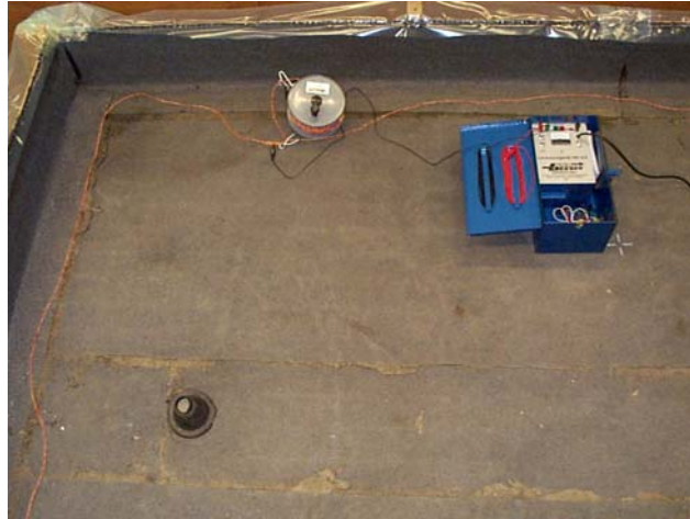
Figure 7: The equipment used for the potential-difference method on one of the test roof systems.
