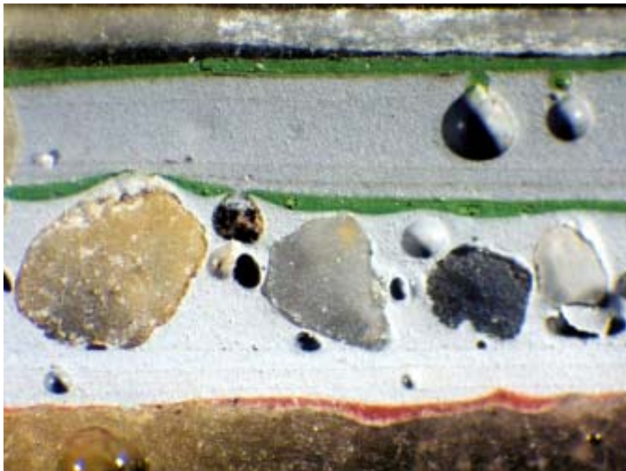
Figure 14 – Photomicrograph of a membrane area with sand particles broadcast into the bottom layer.
