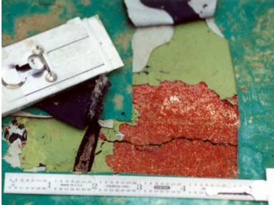
Figure 7 – Interlayer membrane delaminations at various interfaces. Note the substrate crack reflecting through the first light green application of the membrane.
