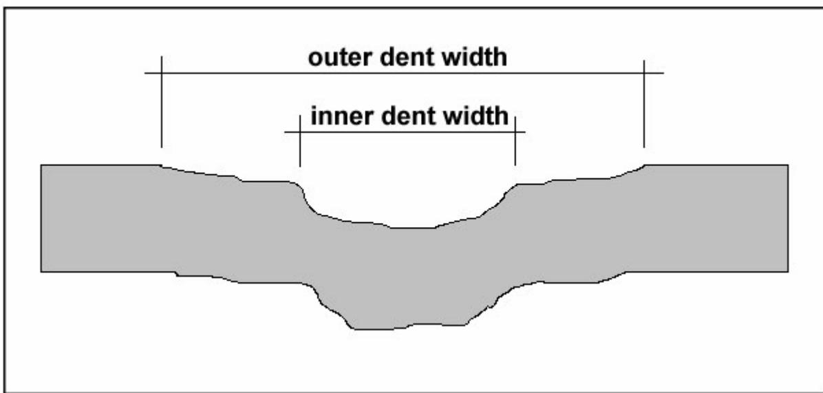
**Figure 12.** Cross section at inner and outer dents in thin-gauge metal.
