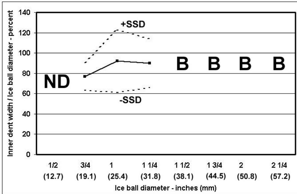
**Figure 15.** Inner dent width versus ice ball diameter for 90-degree impacts against blades of galvanized steel turbine ventilator.
