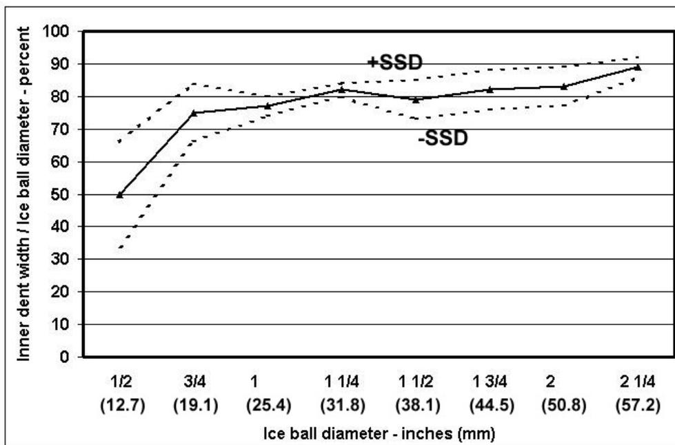
**Figure 22.** Inner dent width versus ice ball diameter for 45-degree impacts against aluminum air-conditioning unit fins.
