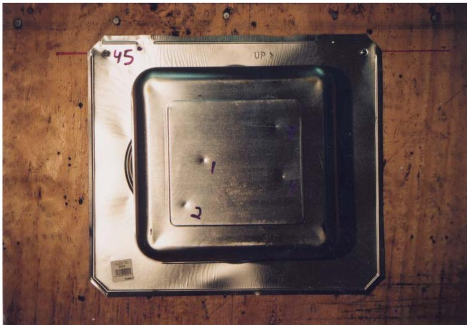
**Figure 10.** Dents in an aluminum static vent from impacts at 45 degrees by 1 1/2-inch- (38.1-mm) diameter ice balls.
