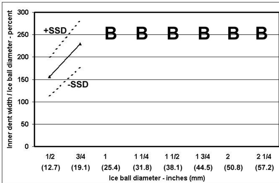
**Figure 18.** Inner dent width versus ice ball diameter for 45-degree impacts against aluminum cover for a water heater combustion products flue.
