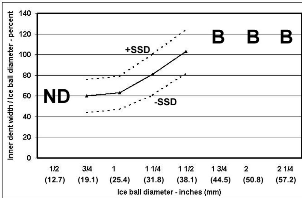
**Figure 16.** Inner dent width versus ice ball diameter for 45-degree impacts against blades of galvanized steel turbine ventilator.
