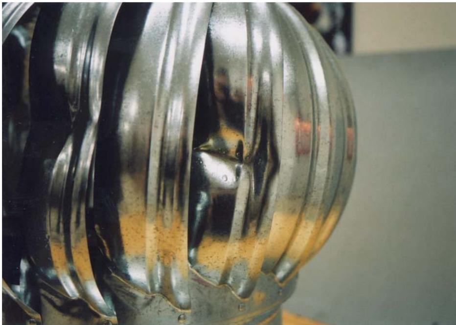
**Figure 8.** Buckle in the blade of a galvanized steel turbine ventilator from impact at 90 degrees by 1 1/2-inch- (38.1-mm) diameter ice ball.
