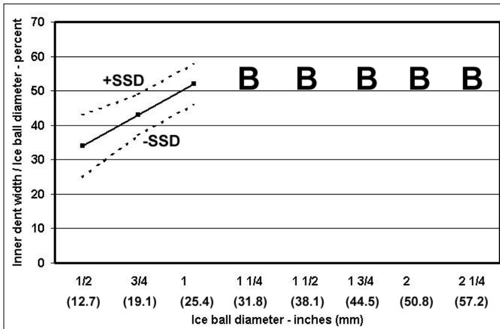
**Figure 19.** Inner dent width versus ice ball diameter for 90-degree impacts against aluminum static vent.
