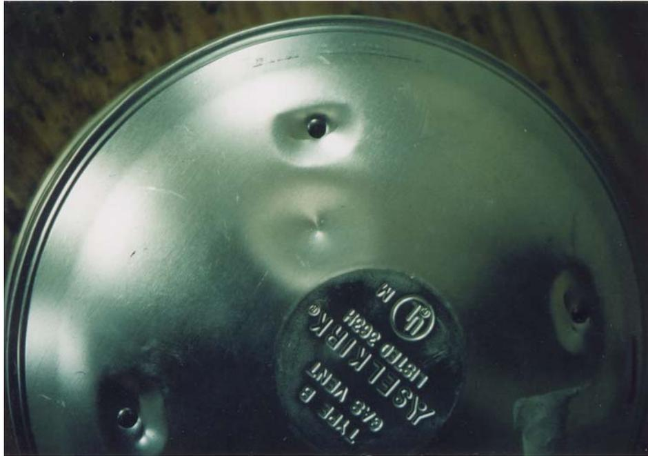
**Figure 9.** Dent in the aluminum cover for a water heater combustion products flue from impact at 90 degrees by 1/2-inch- (12.7-mm) diameter ice ball.
