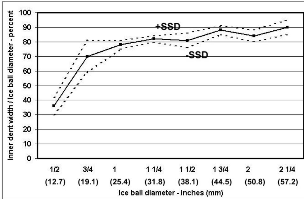
**Figure 21.** Inner dent width versus ice ball diameter for 90-degree impacts against aluminum air-conditioning unit fins.
