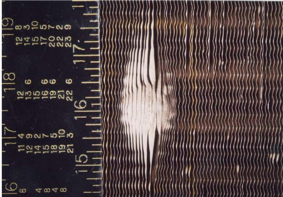
**Figure 11.** Dent in aluminum air-conditioning unit fins from impact at 90 degrees by a 1 1/4-inch- (31.8-mm) diameter ice ball.
