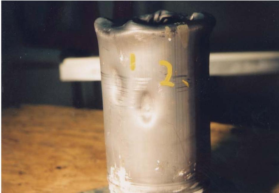
**Figure 7.** Dents in lead soil stack flashing from impacts at 45 degrees by 1 1/4-inch- (31.8-mm) diameter ice balls.
