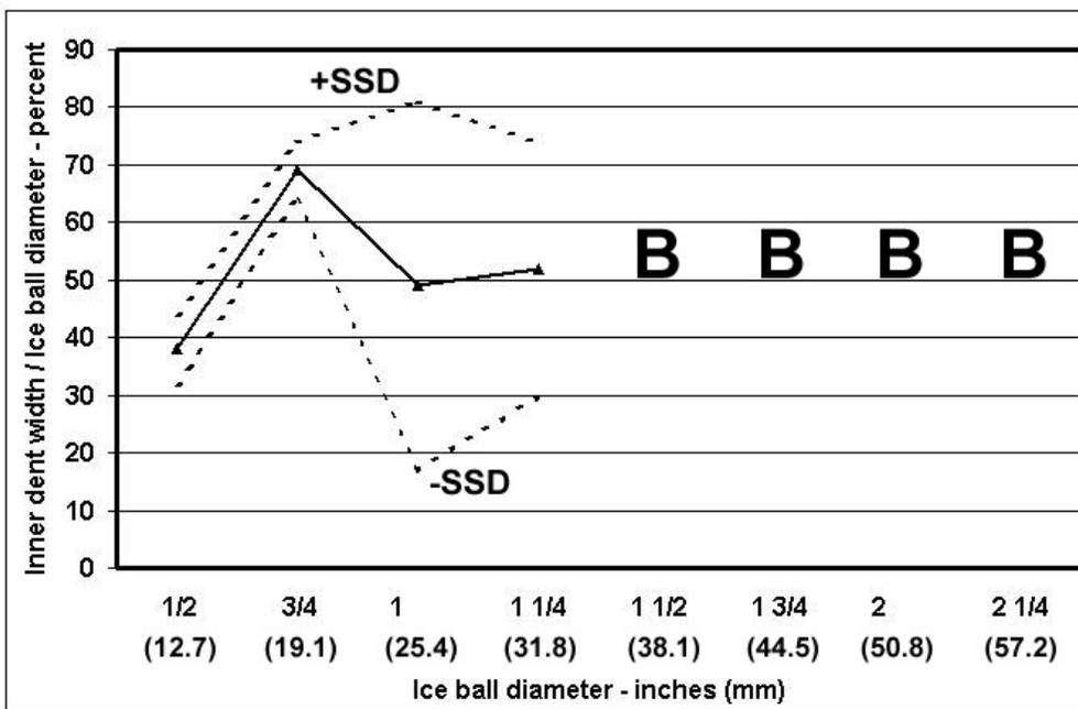
**Figure 20.** Inner dent width versus ice ball diameter for 45-degree impacts against aluminum static vent.
