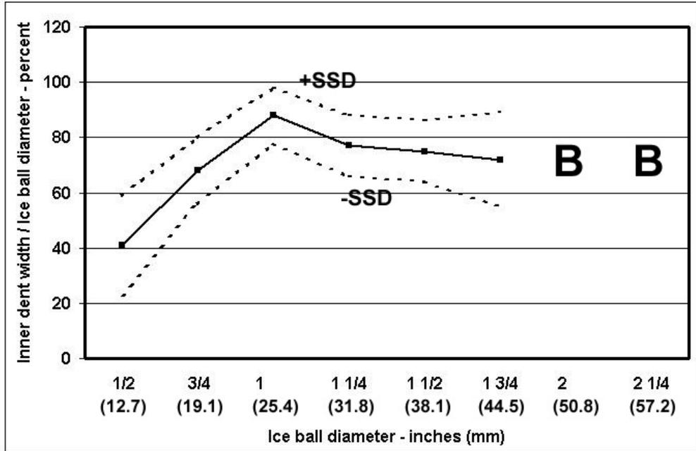
**Figure 13.** Inner dent width versus ice ball diameter for 90-degree impacts against lead soil stack flashing.
