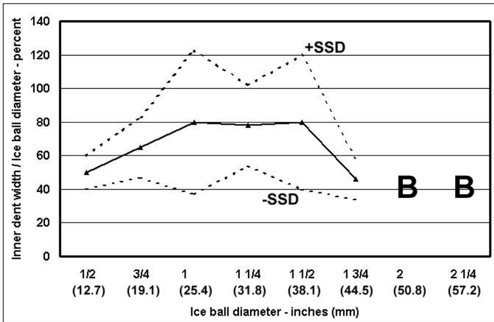
**Figure 14.** Inner dent width versus ice ball diameter for 45-degree impacts against lead soil stack flashing.
