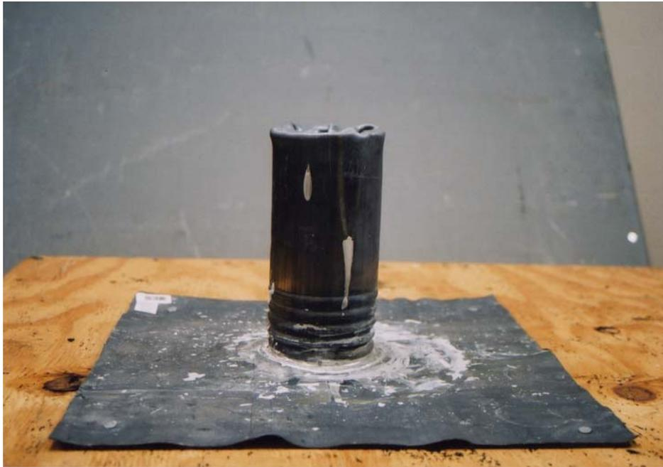
**Figure 1.** Lead soil stack flashing.
