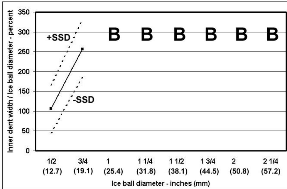
**Figure 17.** Inner dent width versus ice ball diameter for 90-degree impacts against aluminum cover for a water heater combustion products flue.
